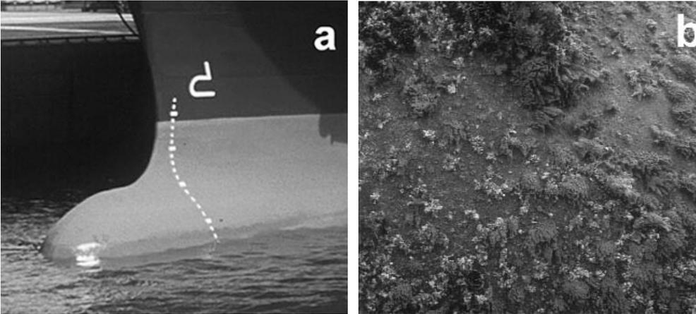
**Fig. 4a-b:** Ships' hull: a) with effective anti-fouling paint containing Tributyltin, b) with ineffective anti-fouling paint and typical clusters of hydroids, barnacles, serpulid worms, and colonies of bryozoa.
